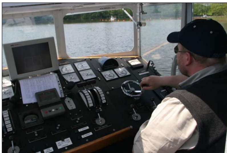
The training model representing a twin CPP ferry. Out-of-window view and control desk located in the wheelhouse.
