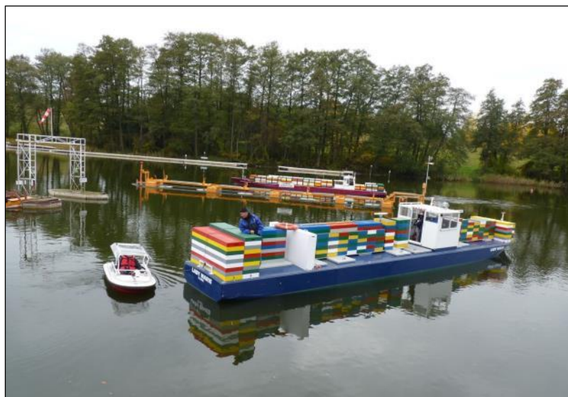
The manned model of an escort tug during a berthing manoeuvre
